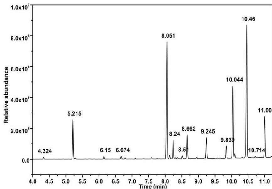
Fig. 3. Fatty acid compounds of microalgal oil analyzed by GC-MS
