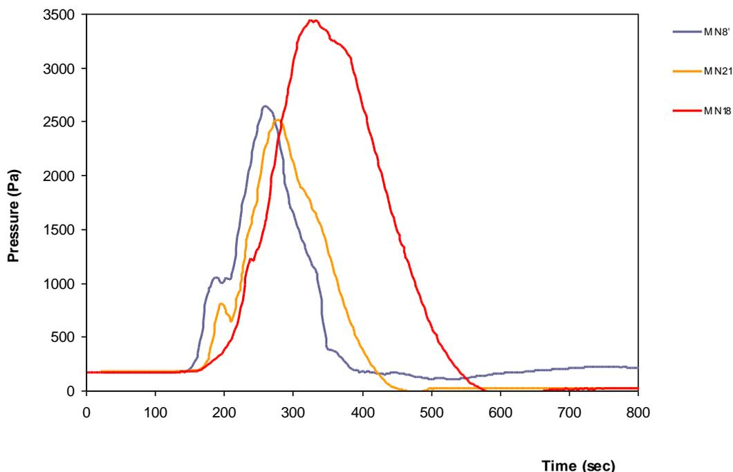
**Fig. 5.** Curves of foam pressure variation as a function of time during foaming for the MN8', MN21, and MN18 foams
