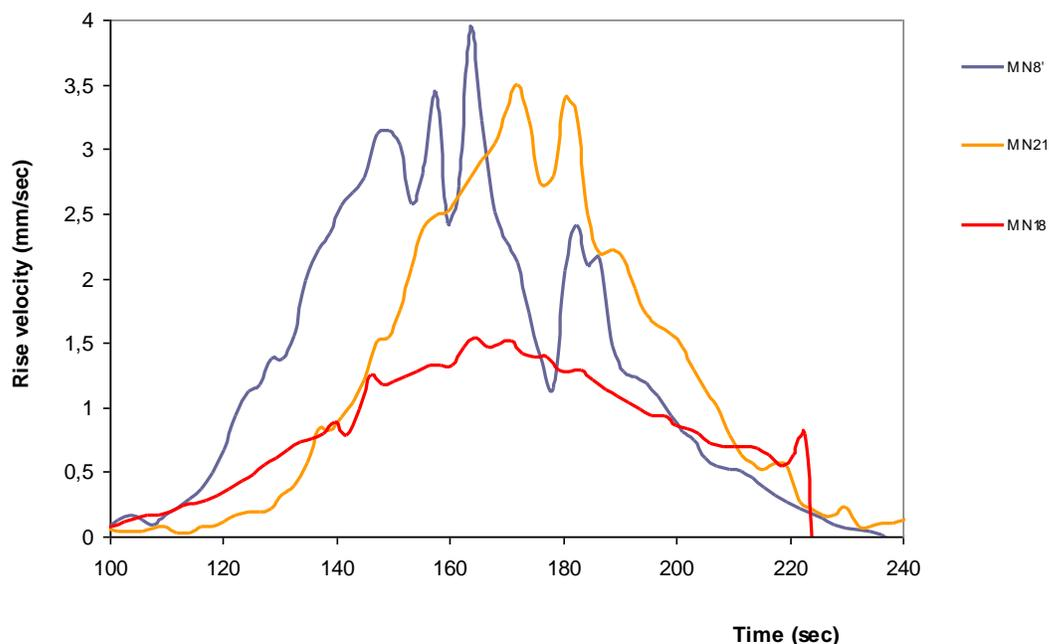
**Fig. 6.** Curves of the velocity of rising foam as a function of time during foaming of the MN8', MN21, and MN18 foams
