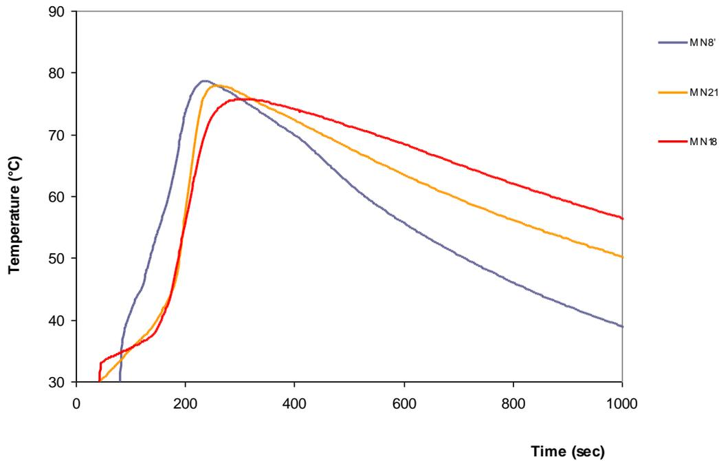
**Fig. 2.** Curves of temperature variation as a function of time during foaming for the MN8', MN21, and MN18 foams
