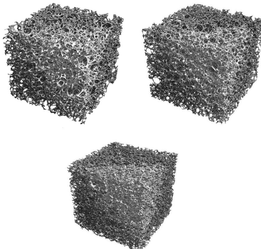
**Fig. 4.** Tomography of (a) MN18 foam, (b) MN21 foam, and (c) MN8' foam. Note the marked differences in structure and cells size among the three foams.
