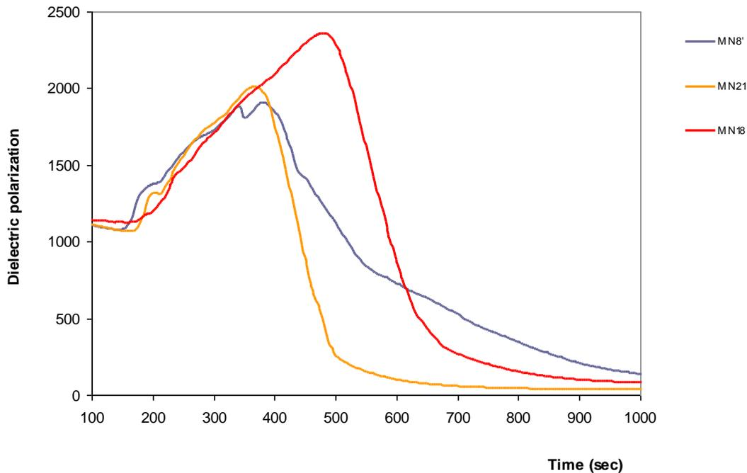
**Fig. 3.** Curves of variation of the dielectric polarization as a function of time during foaming for the MN8', MN21, and MN18 foams
