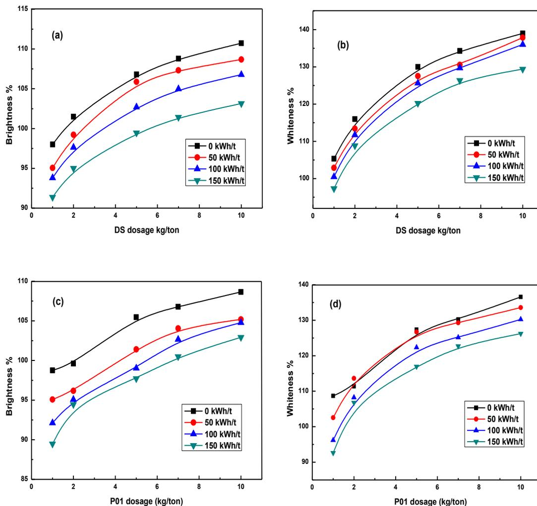
**Fig. 5.** Effect of DS (a, b) and P01 (c, d) on the brightness and whiteness of pulp samples
