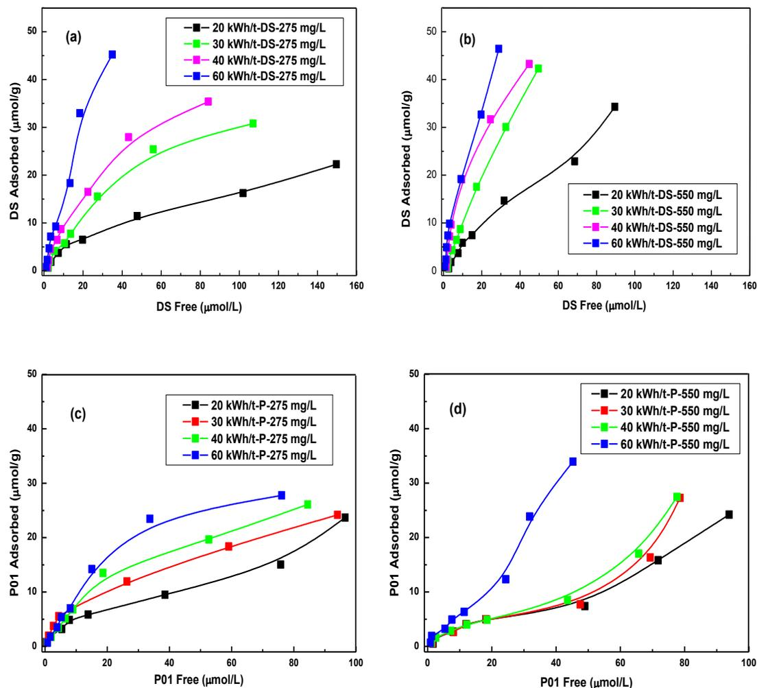
Fig. 8. DS/P01 absorption on eucalyptus pulp with Ca addition before refining
