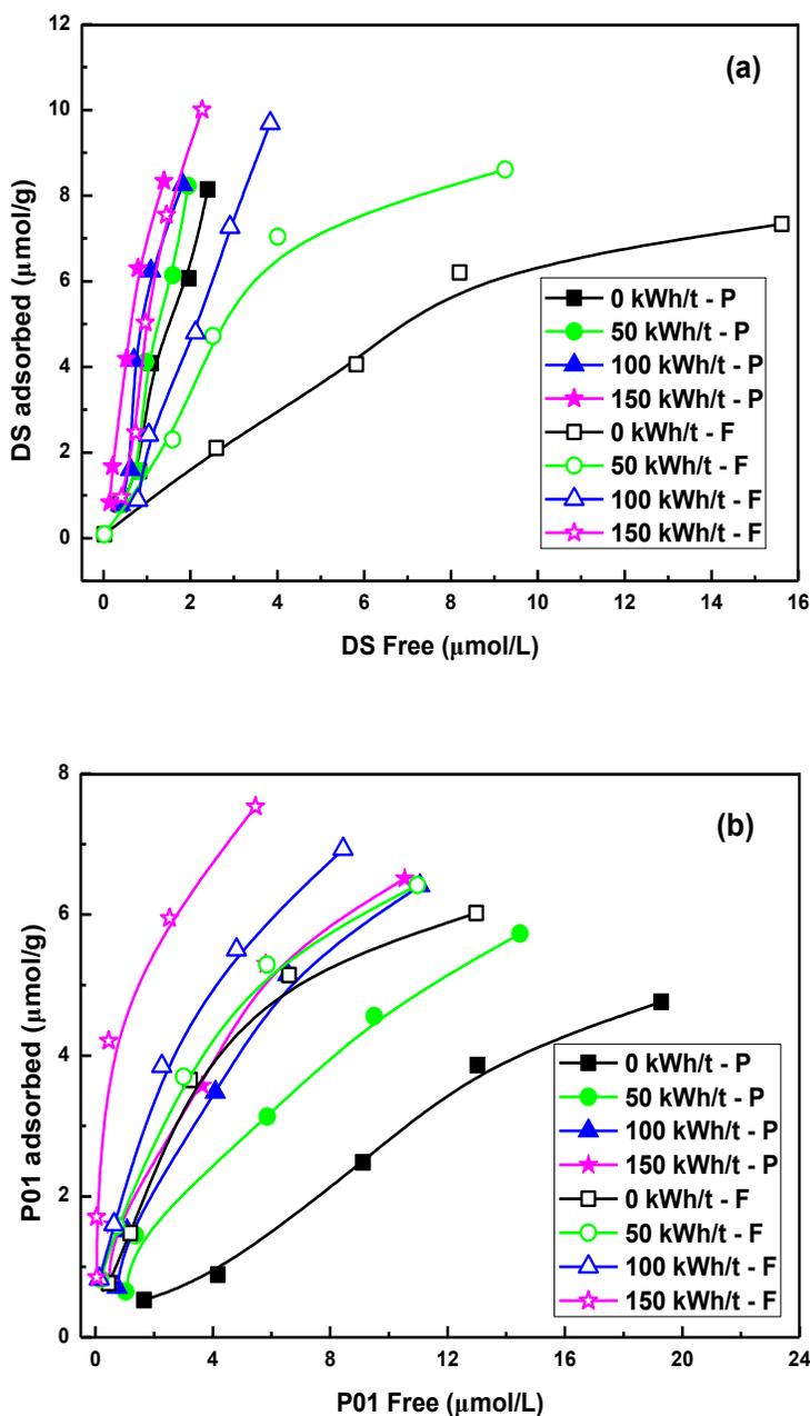
**Fig. 4.** The adsorption of DS (a) and P01 (b) on refined pulp and fiber samples with different SEC levels
