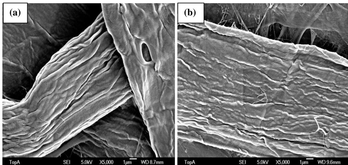
**Fig. 2.** Fiber samples at an FE-SEM magnification 5,000 $\times$ , for (a) 0 kWh/t and (b) 100 kWh/t
