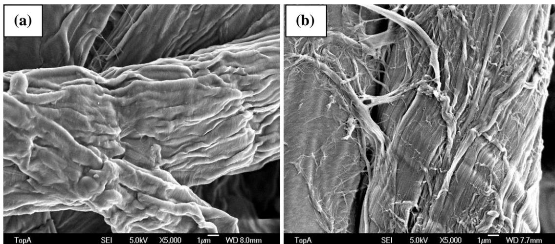
**Fig. 1.** Pulp samples at an FE-SEM magnification 5,000 $\times$ , for (a) 0 kWh/t and (b) 100 kWh/t
