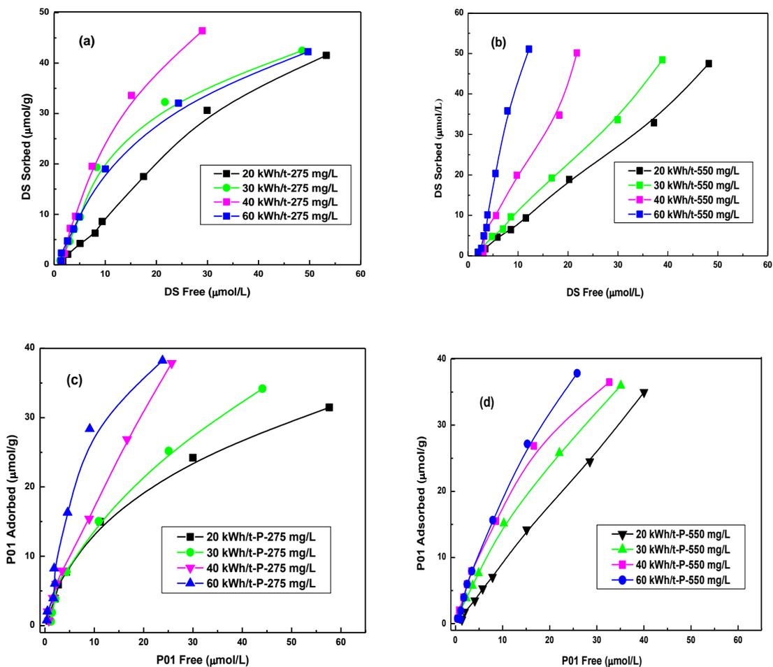
Fig. 7. The adsorption of DS (a, b) and P01 (c, d) on pulp with  $\text{CaSO}_4$  addition after refining
