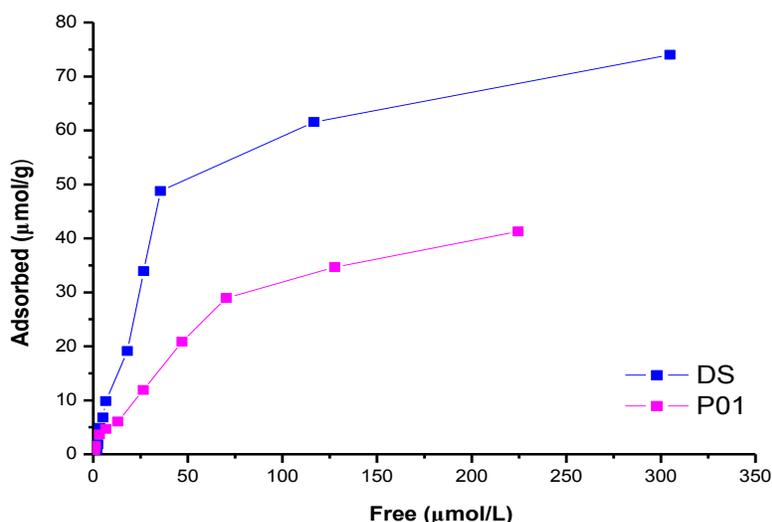
Fig. 3. Adsorption isotherm for FWAs onto reference eucalyptus pulp
