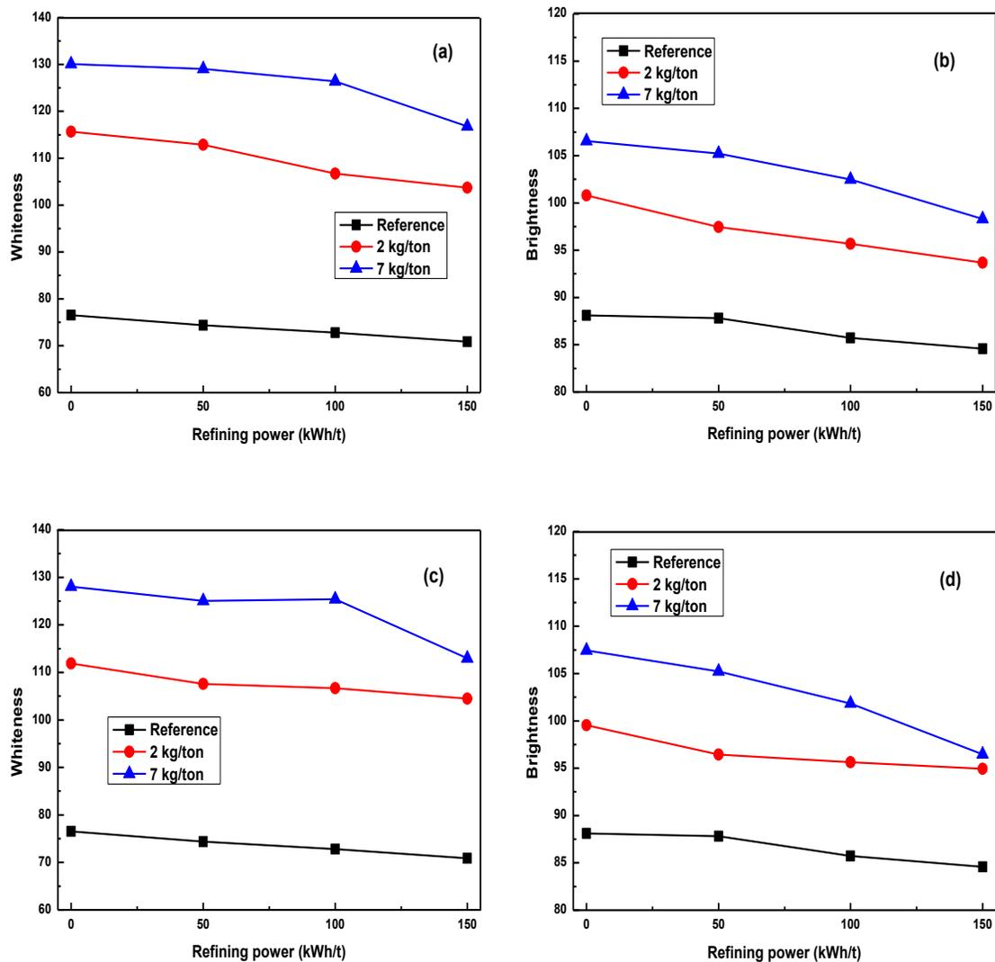
**Fig. 6.** The effect of DS (a, b) and P01 (c, d) addition before refining on the whiteness and brightness of pulp samples
