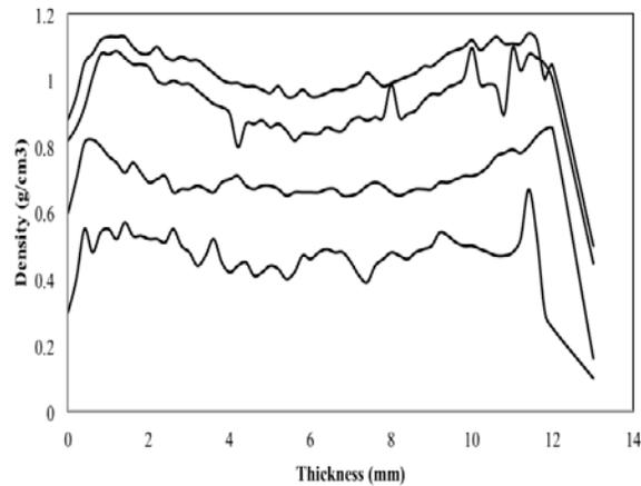
**Fig. 3.** Typical vertical density distribution of hot-pressed natural fiber composites with highly compacted fact and less-highly compacted core
