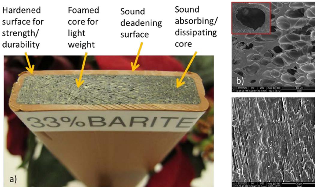
**Fig. 6.** Co-extruded wood plastic composites (WPCs). a) Core-shell structured WPC for sound insulation applications; b) microstructure of foamed WPC core (density=0.55 g/cm<sup>3</sup>), and c) microstructure of unfoamed WPC core (density=1.05 g/cm<sup>3</sup>). Photographs taken by Q. Wu.
