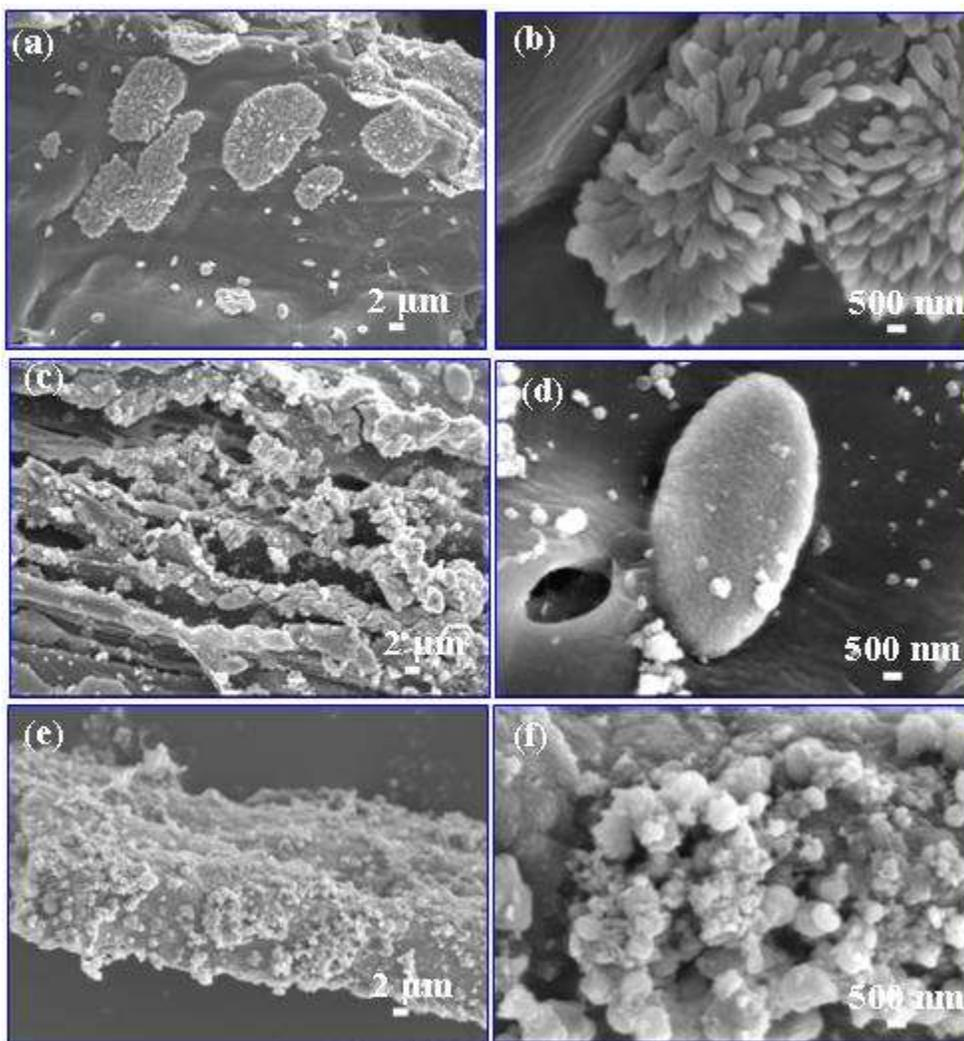
**Fig. 3.** SEM images of the  $\text{CaCO}_3$  particles-filled wood powder nanocomposites: (a, b) 10 min; (c, d) 30 min; and (e, f) 60 min
