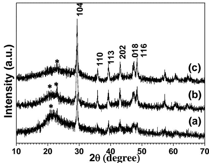
**Fig. 1.** XRD patterns of the  $\text{CaCO}_3$  particles-filled wood powder nanocomposites prepared by microwave heating at  $90\text{ }^\circ\text{C}$  for different times: (a) 10 min; (b) 30 min; and (c) 60 min
