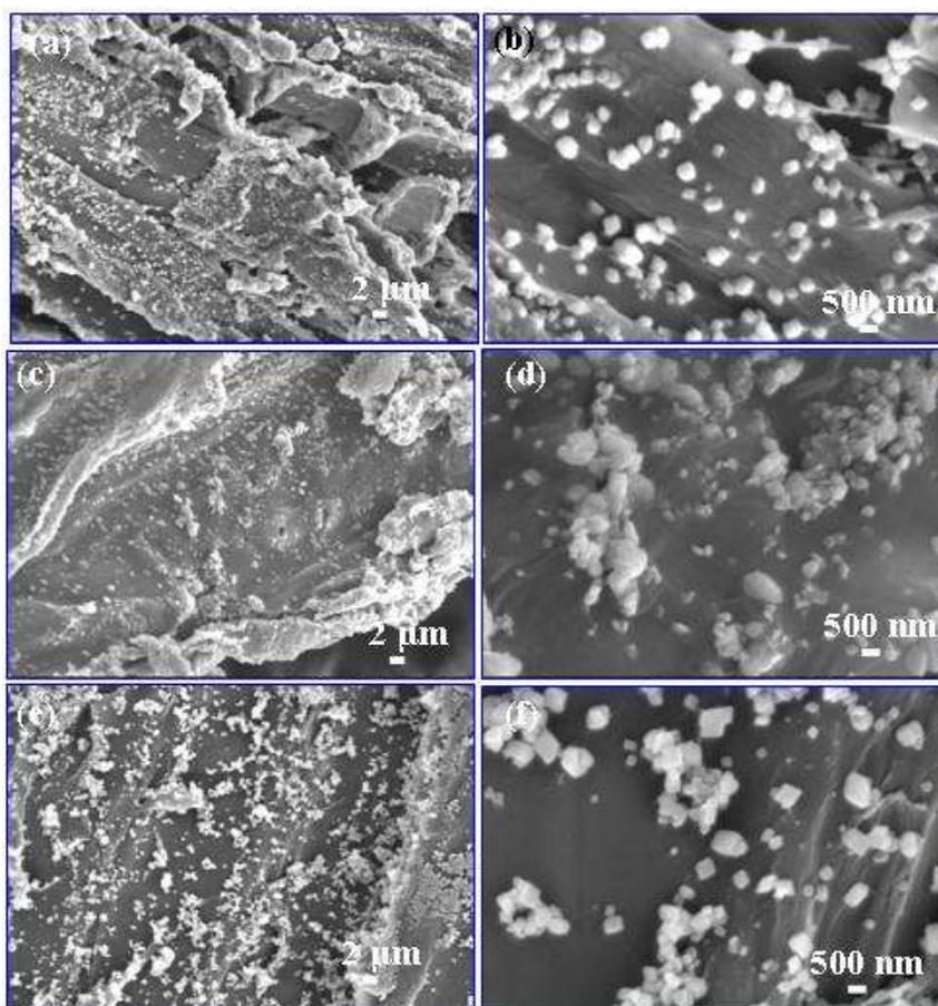
**Fig. 5.** SEM images of the  $\text{CaCO}_3$  particles filled wood powder nanocomposites in the presence of  $(\text{NH}_4)_2\text{SO}_4$  at  $90^\circ\text{C}$  for different times: (a, b) 10 min; (c, d) 30 min; and (e, f) 60 min.
