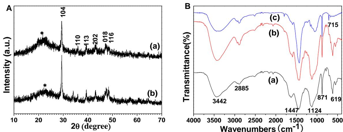
**Fig. 4.** (A) XRD patterns and (B) FTIR spectra of the  $\text{CaCO}_3$  particles-filled wood powder nanocomposites in the presence of  $(\text{NH}_4)_2\text{SO}_4$  at  $90\text{ }^\circ\text{C}$  for different times: (a) 10 min; (b) 30 min; and (c) 60 min
