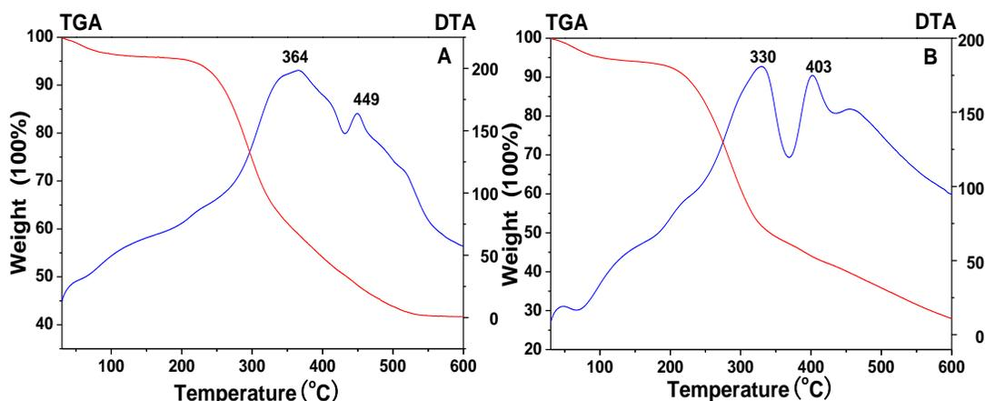
**Fig. 6.** TGA and DTA curves of the  $\text{CaCO}_3$  particles-filled wood powder nanocomposites in the presence of (A)  $\text{Na}_2\text{CO}_3$  and (B)  $(\text{NH}_4)_2\text{SO}_4$  at  $90^\circ\text{C}$  for 30 min.
