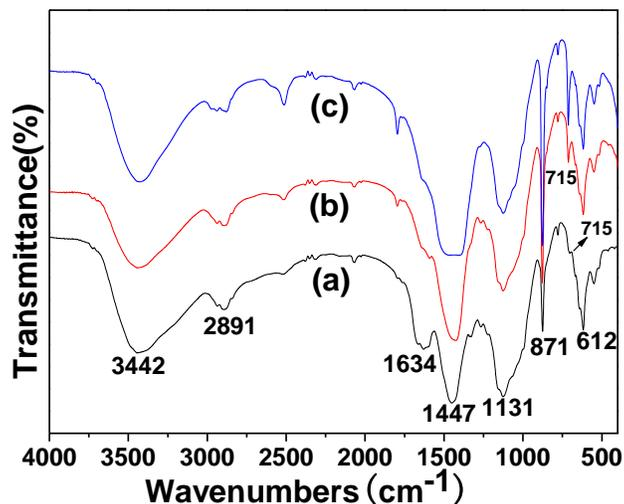
**Fig. 2.** FTIR spectra of the  $\text{CaCO}_3$  particles-filled wood powder nanocomposites: (a) 10 min; (b) 30 min; and (c) 60 min
