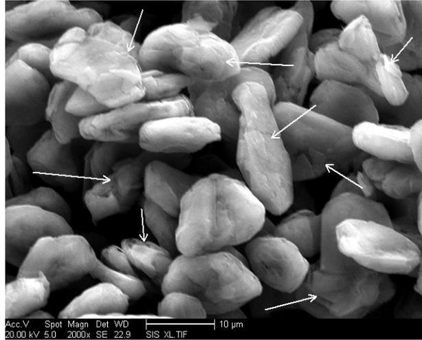
**Fig. 1.** SEM image of natural graphite
