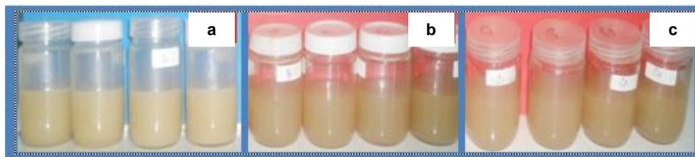
**Fig. 3.** Appearance of gutta-percha-based adhesive at various ratios of gutta-percha to toluene; (a) UGP; (b) GPM; and (c) GPMB
