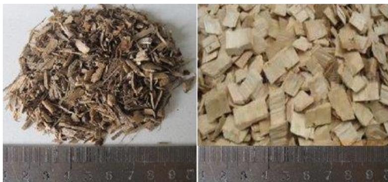
Fig. 1. Morphology of wood pulp wastes (left) and chips (right)
