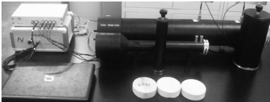
**Fig. 1.** Impedance tubes and samples
