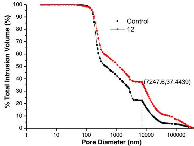
**Fig. 8.** Percentage of intrusion volume versus pore diameter of MW-Treated and control group
