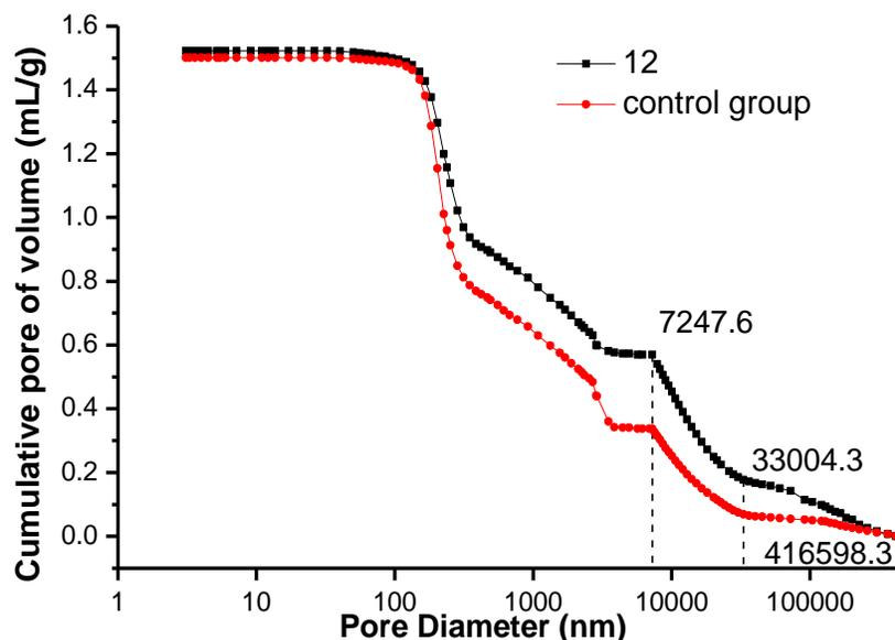
**Fig. 7.** Cumulative pore volume as a function of the pore diameter of wood before and after MW treatment
