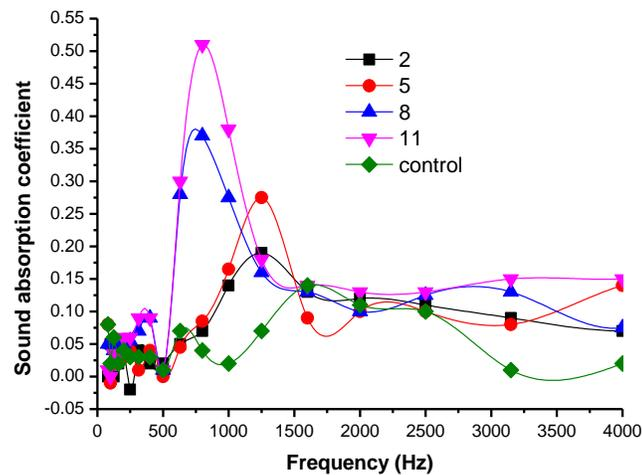
**Fig. 2.** Sound absorption coefficient for treatment wood of different thicknesses
