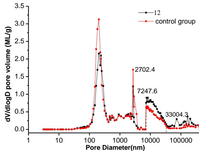
**Fig. 9.** Log differential intrusion as a function of the pore diameter of wood before and after MW treatment
