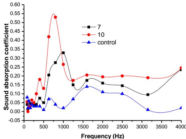
Fig. 3. Sound absorption coefficient at different microwave intensity
