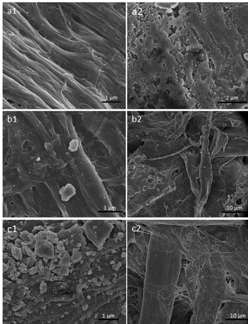
**Fig. 3.** SEM images of the (a1) center and (a2) edge areas of untreated cellulose paper; (b1) center and (b2) edge areas of APTMS-modified paper; (c1) center and (c2) edge areas of chitosan-modified paper. All the papers were loaded with QDs particles for SEM tests.
