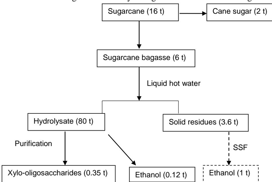
**Fig. 4.** Flow chart of xylo-oligosaccharides and ethanol production from sugarcane bagasse
