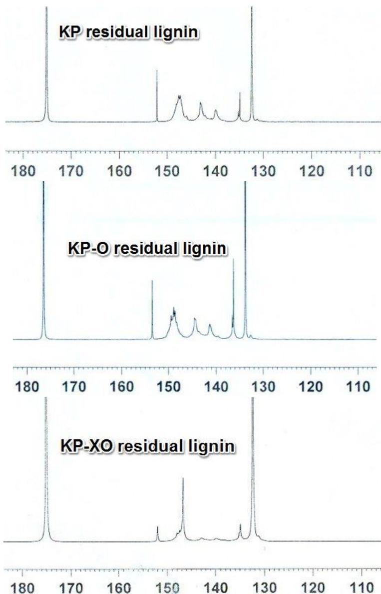
**Fig. 1.**  $^{31}\text{P}$ -NMR spectra of residual lignin (KP is kraft pulp, KP-O is oxygen-delignified kraft pulp and KP-XO is xylanase-assisted oxygen-delignified kraft pulp)
