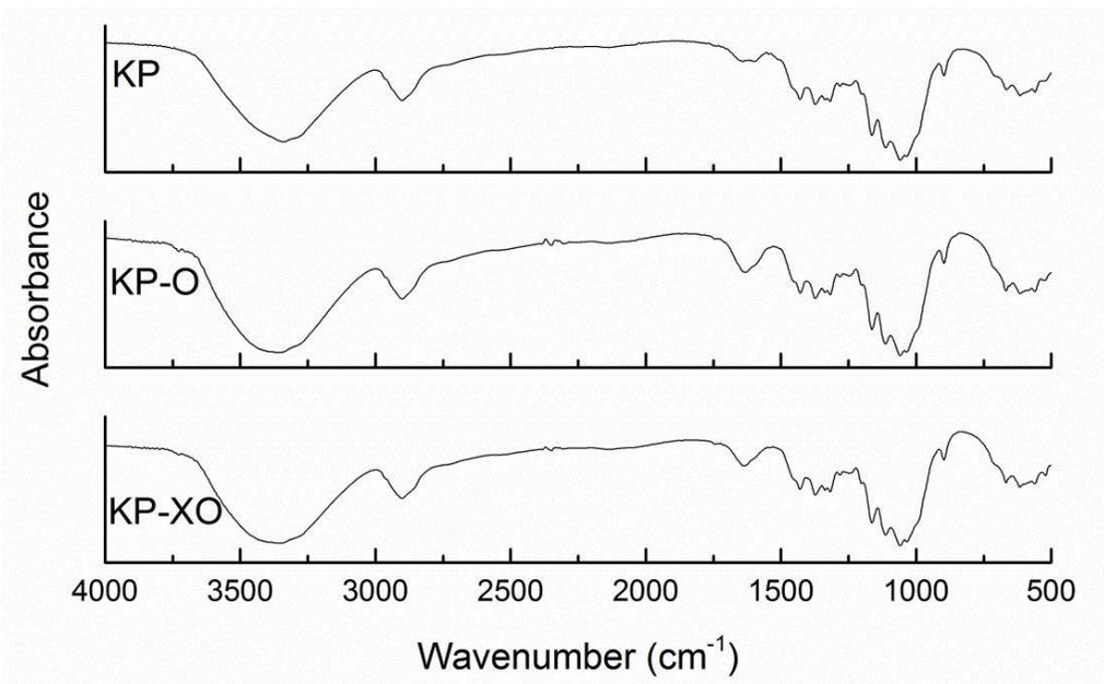
**Fig. 2.** FTIR spectra of kraft pulp and treated pulps
