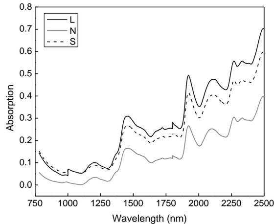
**Fig. 1.** The mean spectra from original data of large knots (L), small knots (S), and knot-free samples (N)
