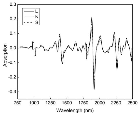
**Fig. 2.** The mean spectra from second-derivative spectra of large knots (L), small knots (S), and knot-free samples (N)
