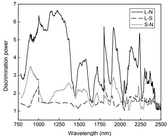
**Fig. 5.** Discrimination power spectra according to SIMCA classification analysis between large knots and normal wood (L-N), between large knots and small knots (L-S), and between small knots and normal wood (S-N)
