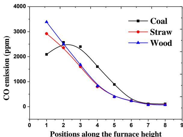
Fig. 2. Axial CO concentration profiles of coal/straw/wood combustion
