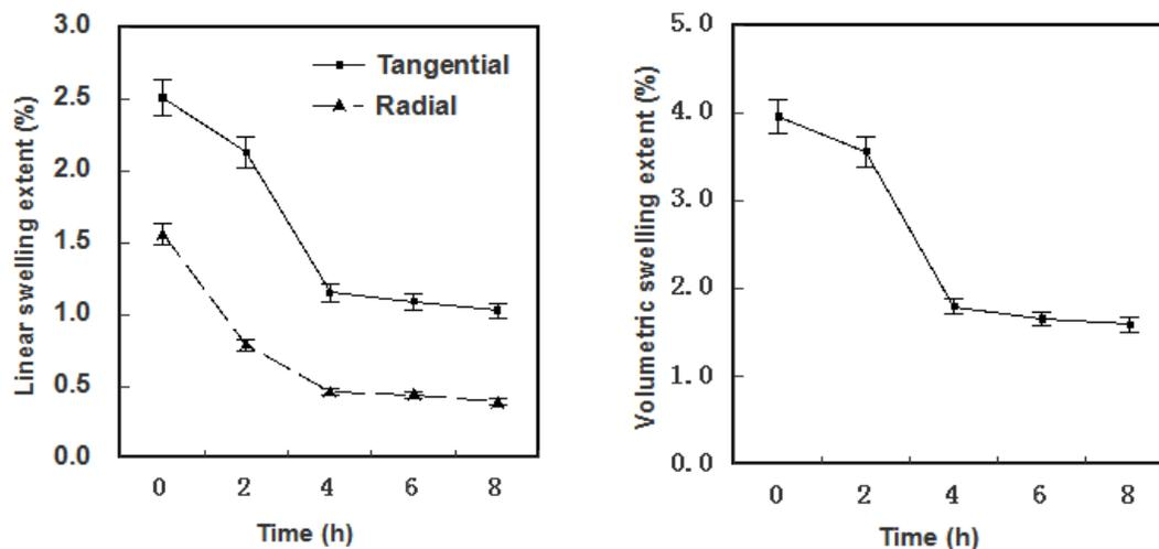
**Fig. 3.** Relationship between wax impregnation treatment time and (a) linear and (b) volumetric swelling extents.
