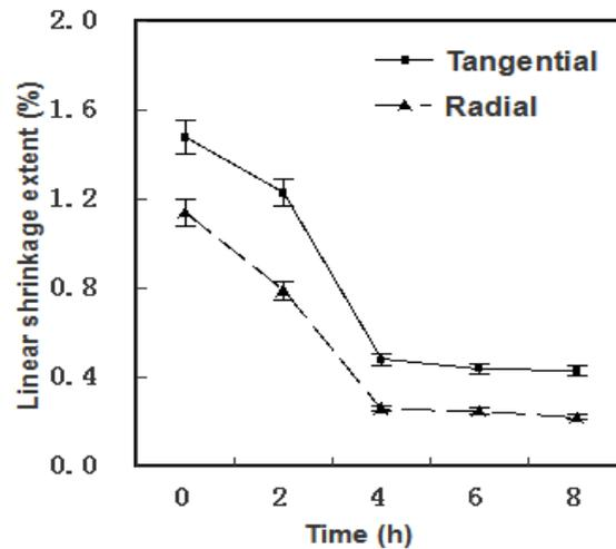
**Fig. 4.** Relationship between the impregnation treatment time and the linear shrinkage extent
