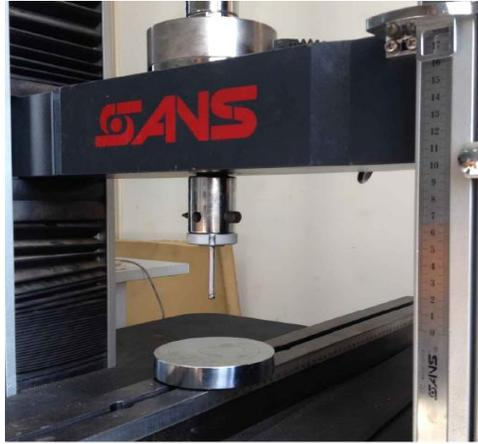
Fig. 1. Surface hardness measurement with WDW-50 hardness testing machine.
