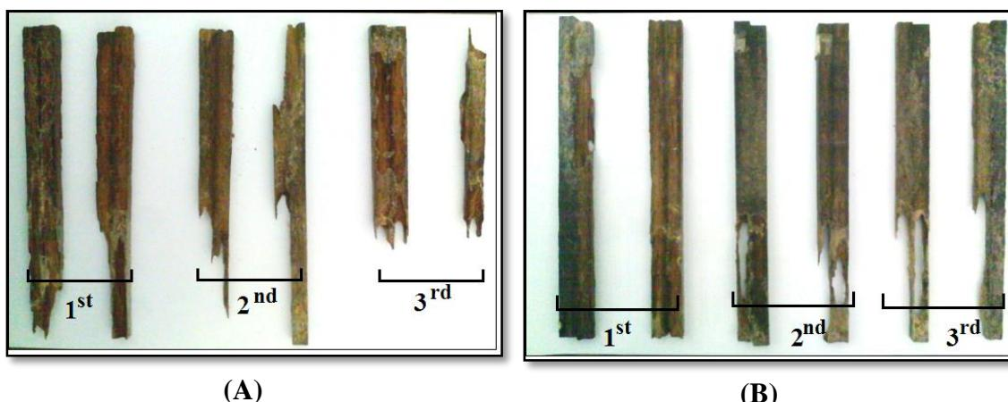
**Fig. 2.** Soil burial tests of compressed OPT samples retained after the 1<sup>st</sup>, 2<sup>nd</sup>, and 3<sup>rd</sup> months.
