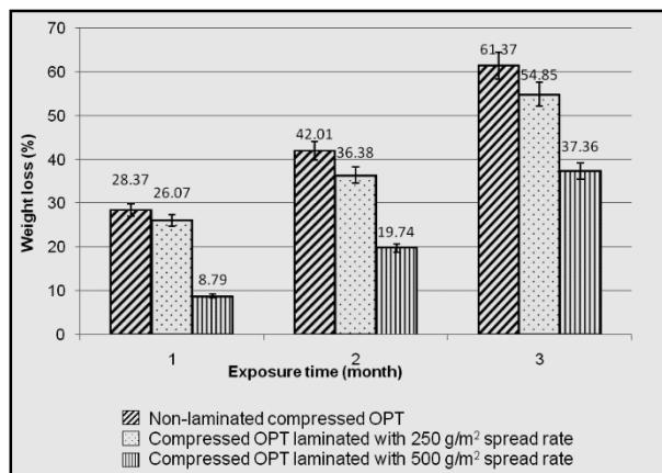
**Fig. 1.** Percentage weight loss of laminated and non-laminated compressed OPT
