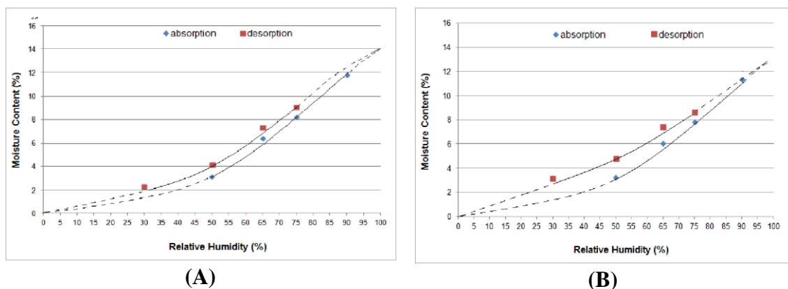
**Fig. 5.** Absorption and desorption curves of compressed OPT: (A) laminated with 250 g/m<sup>2</sup> adhesive spread rate, (B) laminated with 500 g/m<sup>2</sup> adhesive spread rate
