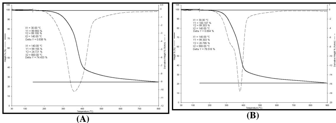
**Fig. 4.** Thermogravimetric analysis curves: (A) compressed OPT without steam pretreatment, (B) compressed OPT with steam pretreatment
