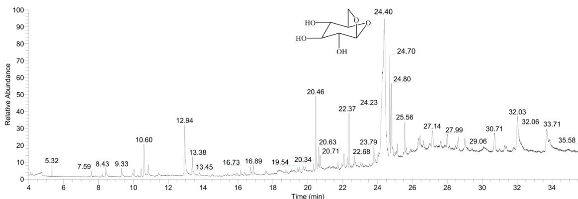
Fig. 6. Ion chromatogram of sugar fraction
