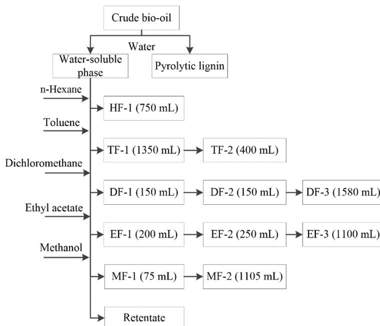
Fig. 1. Column-chromatography separation of bio-oil
