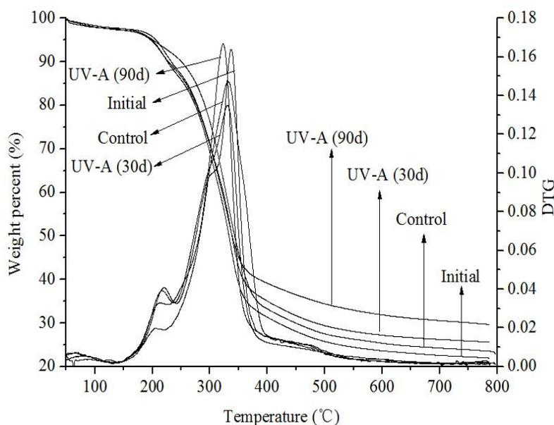
**Fig. 7.** Thermogravimetric analysis of initial, control, and irradiated rice straw. The temperature rate was 25 °C/min.
