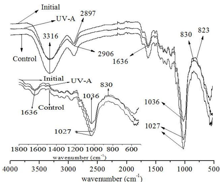
**Fig. 8.** Infrared spectroscopy analysis of initial, control, and treated rice straw samples at day 90
