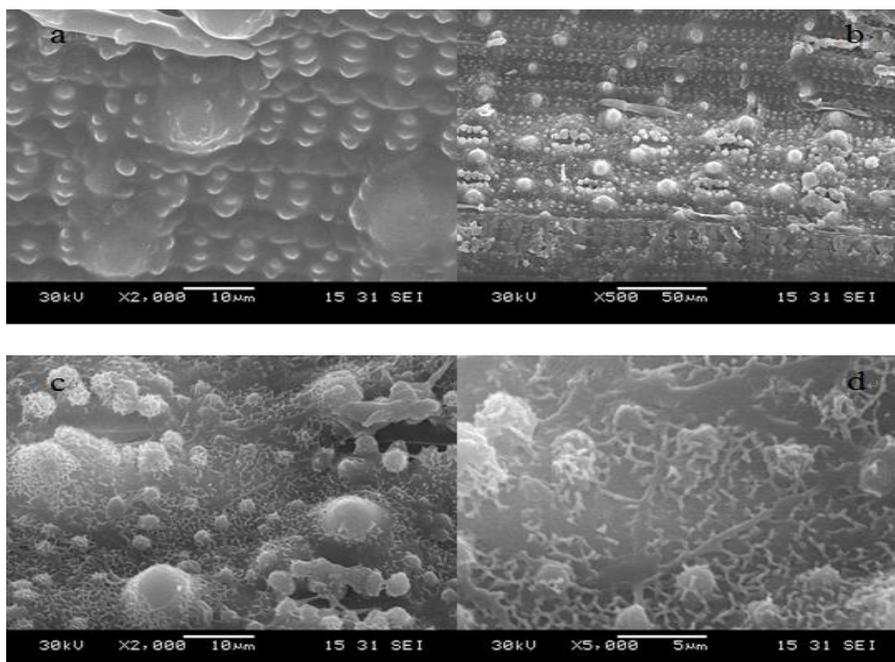
**Fig. 2.** SEM of rice straw surface. (a): initial; (b): sample surface of control at day 90; (c) and (d) refer to irradiated straw surface at day 90
