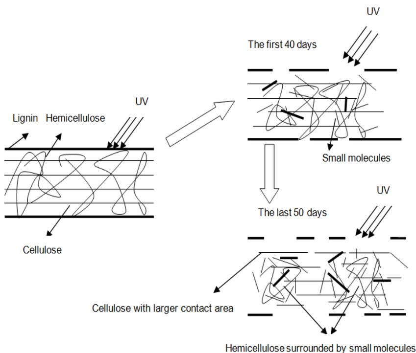
**Fig. 5.** A schematic representation of the effect of UV-A irradiation on lignocellulose at different stage.
