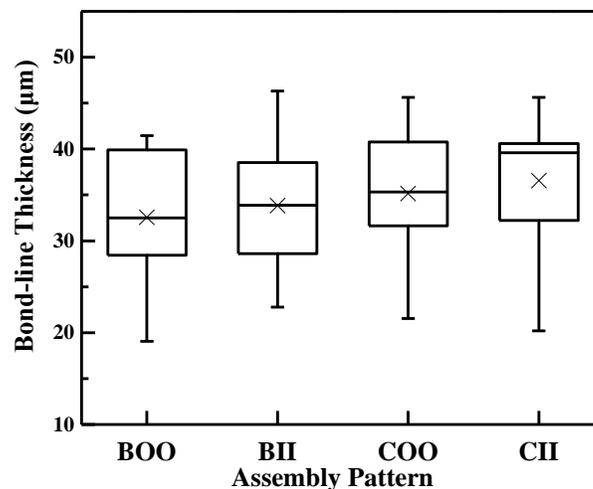
**Fig. 4.** Bond-line thickness of the four kinds of bamboo laminated lumber
