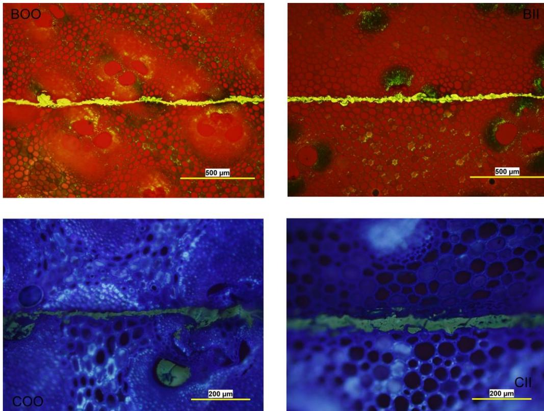
**Fig. 5.** Fluorescent photomicrographs of the four kinds of bamboo laminated lumber
