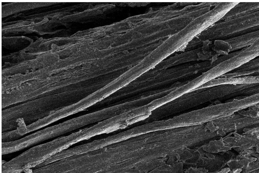
**Fig. 8.** SEM of palm fiber treated with 5% NaOH for 12 h (1000x magnification)
