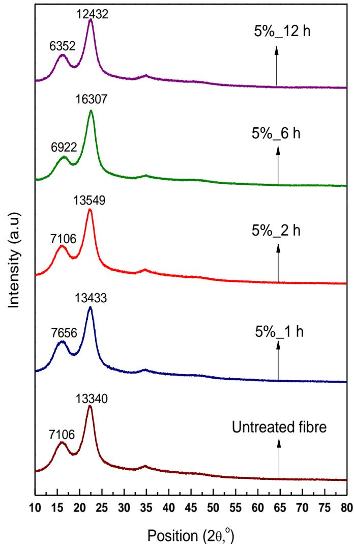
**Fig. 4.** XRD patterns of untreated palm fiber and fiber treated with 5% NaOH for 1, 2, 6, or 12 h
