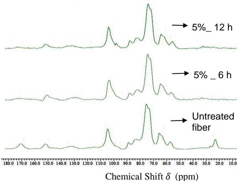
**Fig. 9.** CP/MAS <sup>13</sup>C NMR spectra of raw and alkali treated fiber
