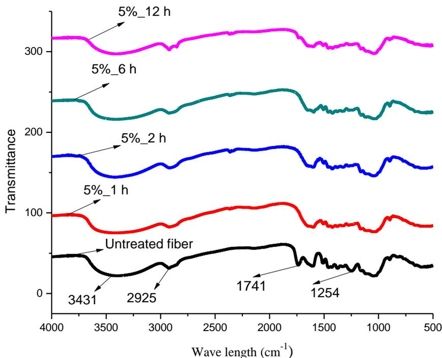
Fig. 5. FTIR spectra of raw and alkali-treated fiber
