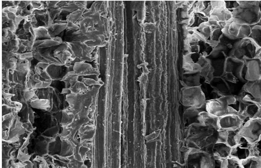
**Fig. 7.** SEM of palm fiber treated with 5% NaOH for 6 h (1000x magnification)
