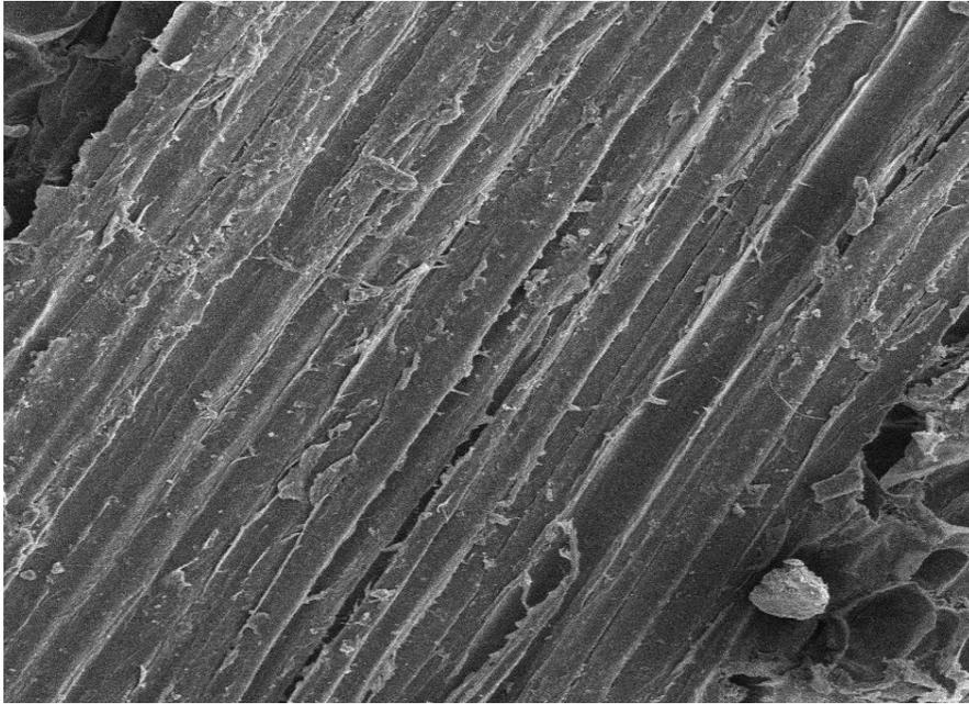
**Fig. 6.** SEM of raw palm fiber (500x magnification)
