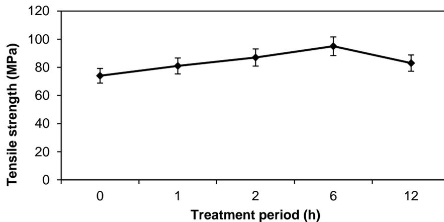
**Fig. 2.** Tensile strength of untreated and treated palm fiber
