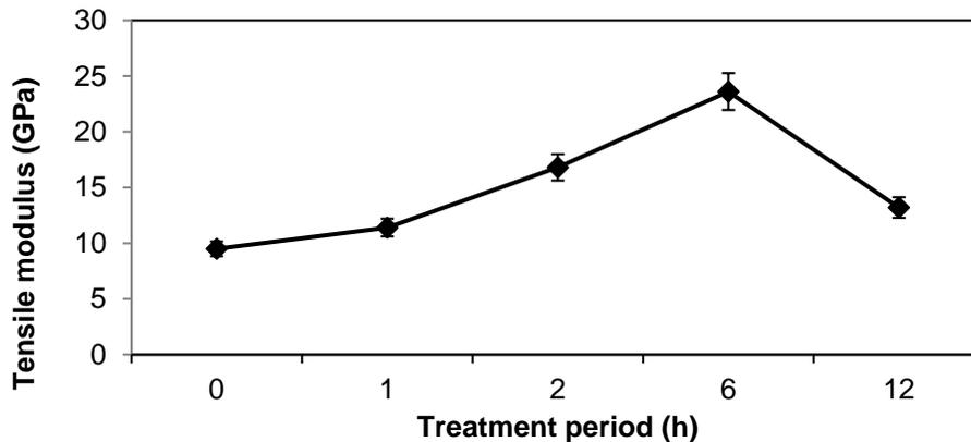
**Fig. 3.** Tensile modulus of untreated and treated palm fiber
