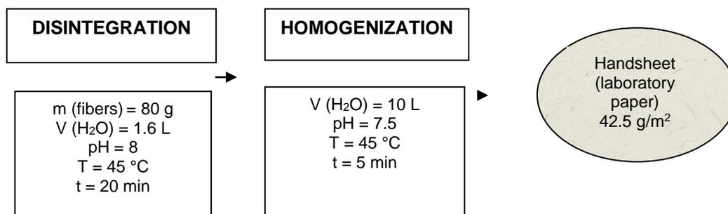
**Fig. 1.** Workflow of laboratory paper production
