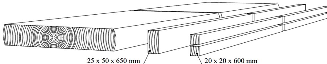
**Fig. 1.** Scheme of preparation of test samples
