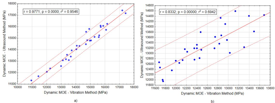
Fig. 6. Correlation between dynamic modulus of elasticity for spruce (a) and oak wood (b)
