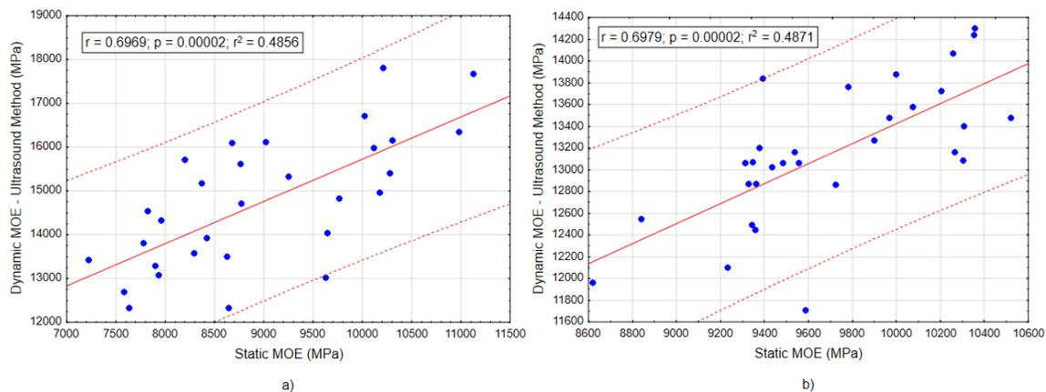
**Fig. 4.** Correlation between  $MOE_{u, 565}$ , measured in 565 mm, and MOEs for spruce (a) and oak wood (b)
