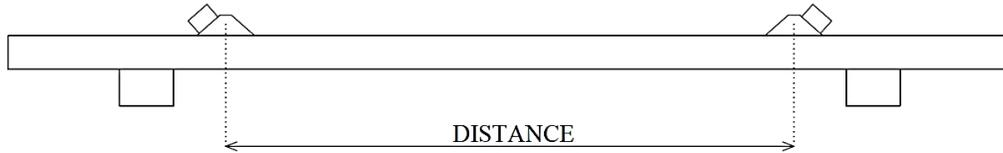
**Fig. 2.** Position of transducers during ultrasound NDT testing
