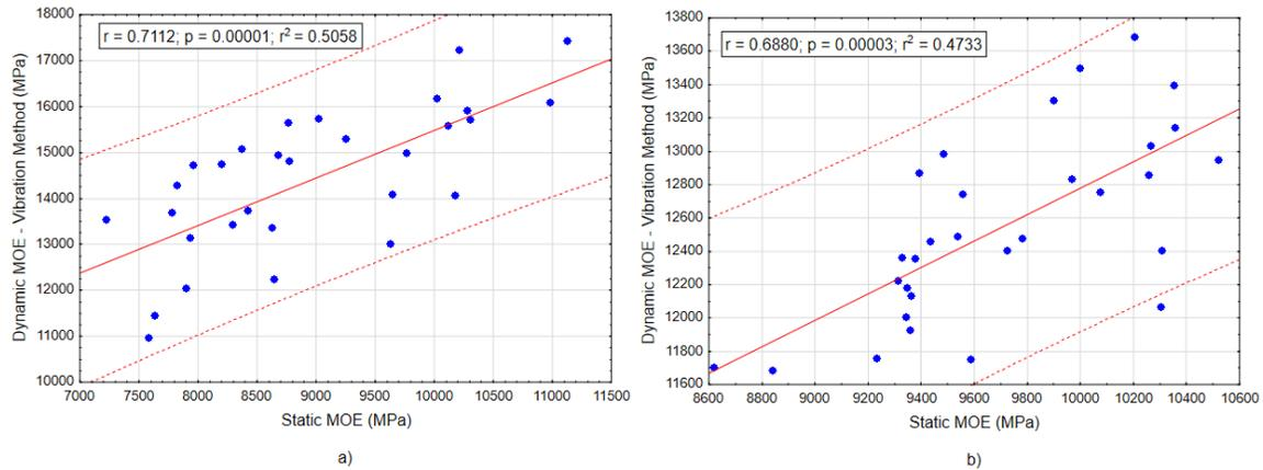
Fig. 5. Correlation between static and dynamic vibration MOE for spruce (a) and oak wood (b)
